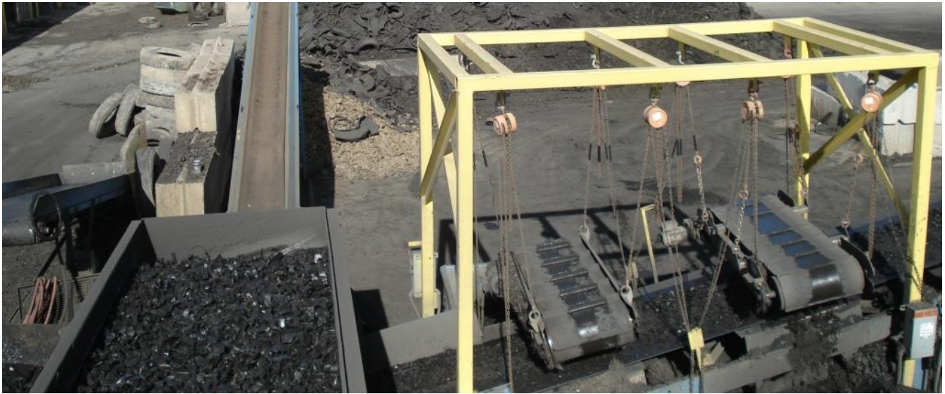
Two belt magnets to the right of the picture removed loose wire at Liberty Tire in Jefferson County. Liberty Tire is the largest supplier of tire derived products in the Commonwealth. (Photographs courtesy of Terry Gray, TAG Resource Recovery, November 2012).
