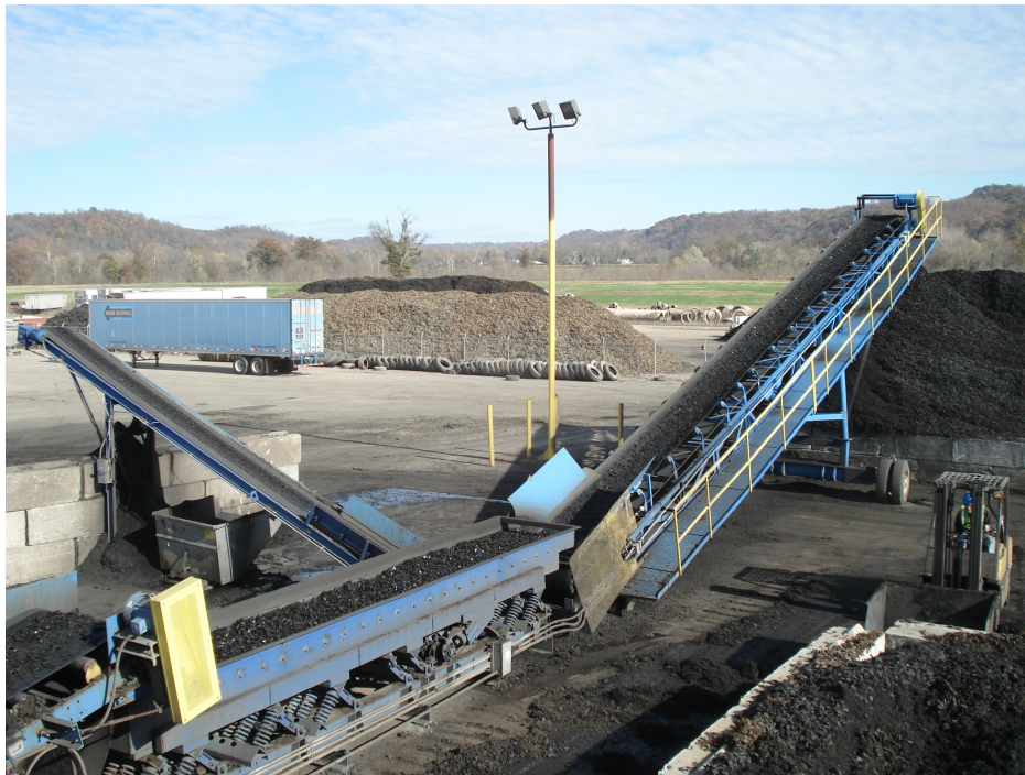
A screen in the left foreground sorts tire chips. Then a conveyor dropped product into a pile at Liberty Tire in Jefferson County. “Fluff” from shredding tires, the fabric material, is in the right foreground. The muddy chips in the background were from the Simpson County tire fire remediation.
